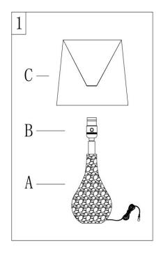
Step1 Place shade(C) onto the Socket(B).
