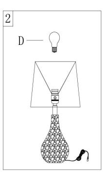
Step 2 Insert the bulb(D) into the socket(B).
