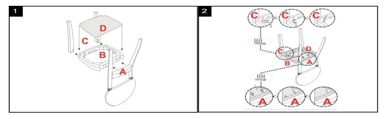
Assembly part A and B first with bolt Nuts M8x60 mm and ring Assembly part C and B first with bolt Nuts M8x60 mm and ring Assembly part D in upper Part B
