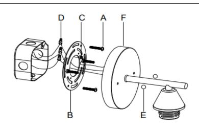
**Step 1:** Secure mounting plate (B) to outlet box with mounting screws (A).
