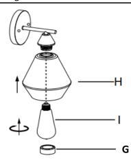
Step 4: Place the glass shade cover (H) on the socket and tighten it clockwise with the socket ring (I) Insert the bulb (G) into the socket.
