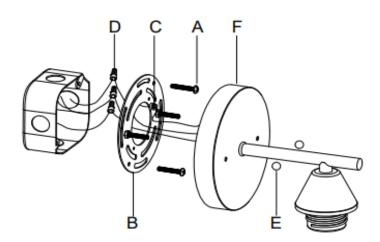
**Step 3:** Attach the Lamp body (F) to the Mounting plate (B) and secure with Round nut €
