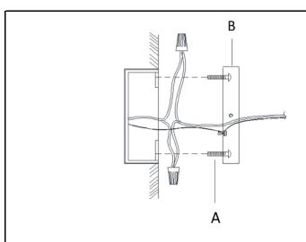
Step 1: Lock back plate (B) to junction box with outlet box screws (A).
