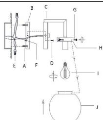
**Step 4:** Lock the bulb (I) to the socket. Lock the glass shade (J) to the lamp cup (H) with 3pcs screws (G).
