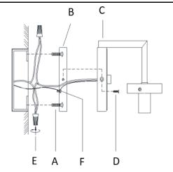
Step 3: Lock fixture body (C) to back plate (B) with mounting screws (D).
