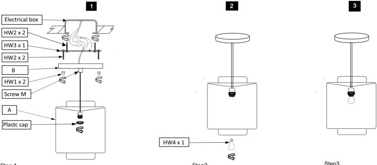
Insert the bulb(HW4) into the Lampholder.
