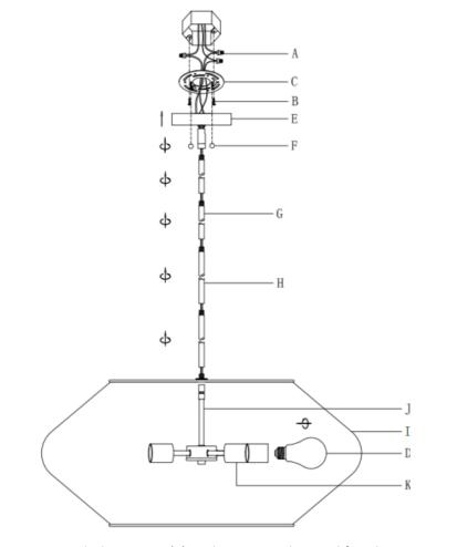
the Canopy Nut(F) clockwise. Insert the bulbs (D) into the Sockets (K).
