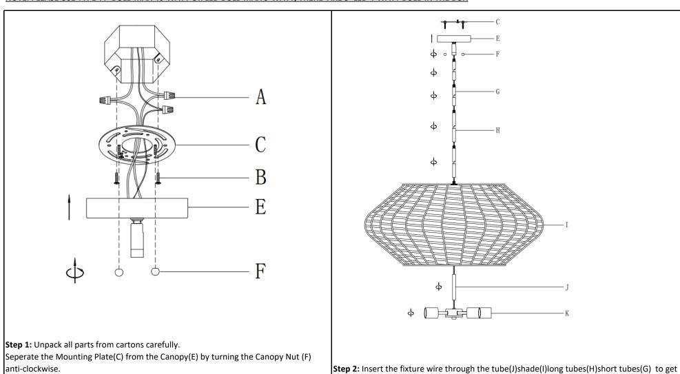
desired length to Canopy(E). then Rotate each part clockwise till tight.
