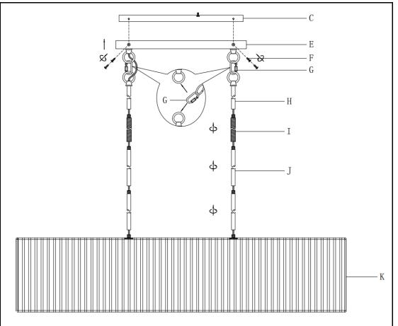
Loop+tube (H) in turn to get desired length. Rotate each part clockwise till tight. Connect Fixture Loop+tube (H) and Canopy(E) with the Closable Link (G).
