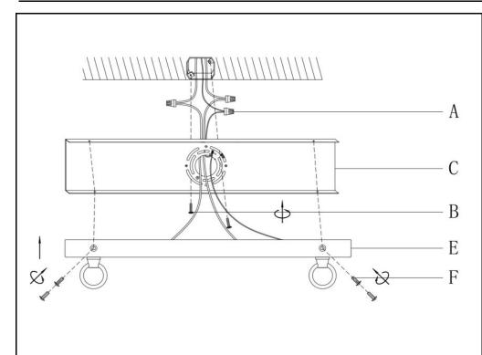
Step 1: Unpack all parts from cartons carefully. Seperate the Mounting Plate(C) from the Canopy(E) by turning the Canopy Screw | Step 2: Insert the fixture wire through the long tubes(J), Twine tube(I), Fixture (F) anti-clockwise. Install the Mounting Plate(C) to the junction box with Mounting Screw (B).
