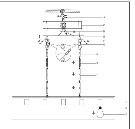
**Step 4:** Attach the Canopy(E) to the junction box and fix it by turning the Canopy Screw(F) clockwise. Insert the bulbs (D) into the Sockets(L).
