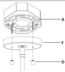
Step 4: Place the canopy assembly (F) over the outlet box, and ensure the heads of the support screws of the mounting bracket (A) come through the holes of the canopy assembly (F). Tighten the cap nuts (D) onto the protruding support screws on the mounting bracket (A) until the canopy assembly (F) is held firmly against the ceiling.
