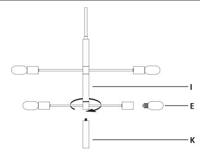
Step 5: Install the light bulbs (E) into the socket of the lamp body (I).
