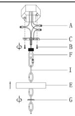
**Step 4:** Install the Mounting Plate(C) to the junction box with Mounting Screw (B).
