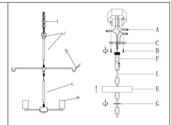
**Step 2:** Screw Fixture Loop (J) to Cross-braces (N) until firmly tightened. Place the Fixture Loop (J) onto the Closable Link (H).
