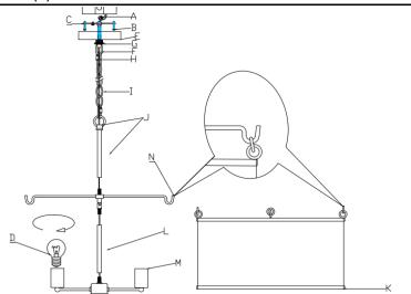
**Step 6:** Pass the wires one by one through (L) (N) (J) and twist them together, and then hang them on Closable Link(H), Insert the bulb (D) into the Socket, Take out the Shade (K). Then hang Cross-braces (N) on the small rings of Shade(K)
