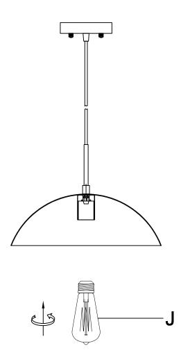
Step 5: Fix the bulb (J) into the lamp holder
