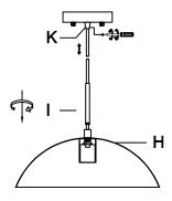
**Step 2**:Rotate the short rod (I) and fix it on the lamp body (H). After loosening the screw in the iron sheet (K), you can adjust the wire up and down to the appropriate position, and then tighten the screw in the iron sheet (K)
