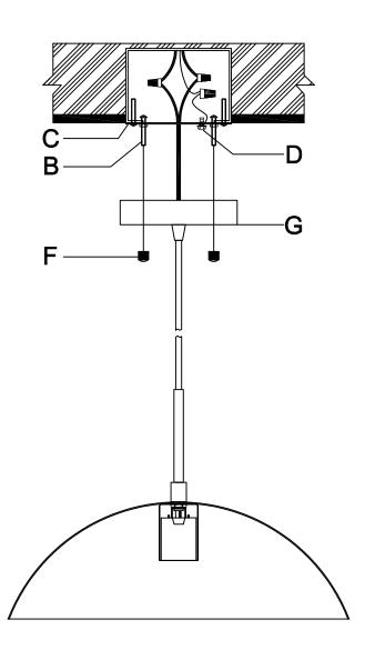
Step 4: Attach the canopy (G) to the Mounting Plate (C),and fix it by turning the canopy nut (F) anti clockwise
