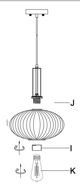
Step 5: Fix the glass (J) on the lamp holder with the lamp shade (I) .and then fix the bulb (K) into the lamp holder
