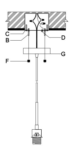
Step 4: Attach the canopy (G) to the Mounting Plate (C), and fix it by turning the canopy nut (F) anti clockwise.
