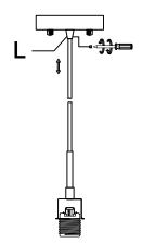
**Step 2**:After loosening the screw in the iron piece (L), you can adjust the wire up and down to a proper position, and then tighten the screw in the iron piece (L).
