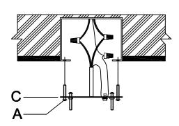
**Step 1**:Unpack all parts from cartons carefully. Fix the Mounting plate (C) to the junction box with machine screw (A)
