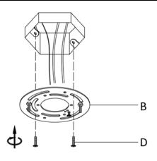
**Step 4:** Fix the Mounting Plate(B) to the junction box with Mounting Screw (D).
