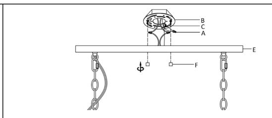
**Step 6:** Tuck wires inside junction box. Attach the Canopy(E) to the Mounting Plate (B), and fix it by turning the Canopy Nut (F) clockwise.
