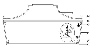
**Step 1:** Unpack all parts from cartons carefully. Attach the ends of the Square Tube Pillars (P) to the Top Square Tube Frame (N) and Bottom Square Tube Frame (Q) with Screw (O). Spread arm of the Arm Assembly (L), attach the Arm Assembly (L) to the Top Square Frame (N) with Ball Screw (M).
