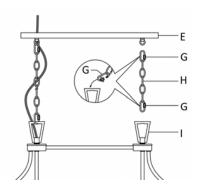
**Step 3:** Use Closable Link (G) attach the Chain (H) ends onto the Fixture Loop (I) and the hanging loop at the bottome of Conapy (G). Gently cord and ground wire through Chain (H) and Canopy (D),through Chain (H) about every third link.
