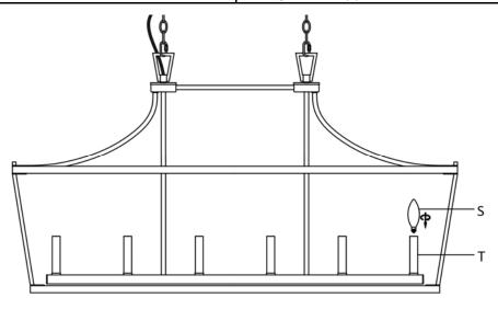
Step 7: Insert the Bulbs (S) into the Sockets
