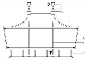
**Step 2:** Thread the Center Rod (R) to the Socket Assembly (T). Attach the Center Rod (R) to the Arm Accembly (L), Cap (K) and Rubber Washer (J), then secure with Fixture Loop (I).
