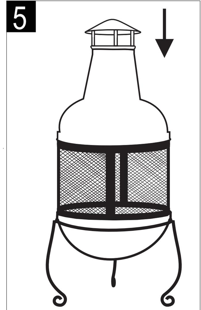
Step 5: Place the cap(C) on the top of the chimni cover .
