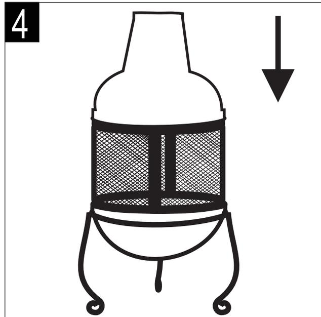
Step 4: Place the chimni cover(CC) on the top of the net
