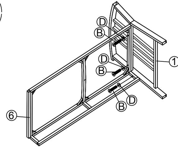
STEP 6: Connect Right Frame (1) & Seat Bench (6), tighten Allen Bolt (B), Flat Washer(D) with Allen Key (E).
