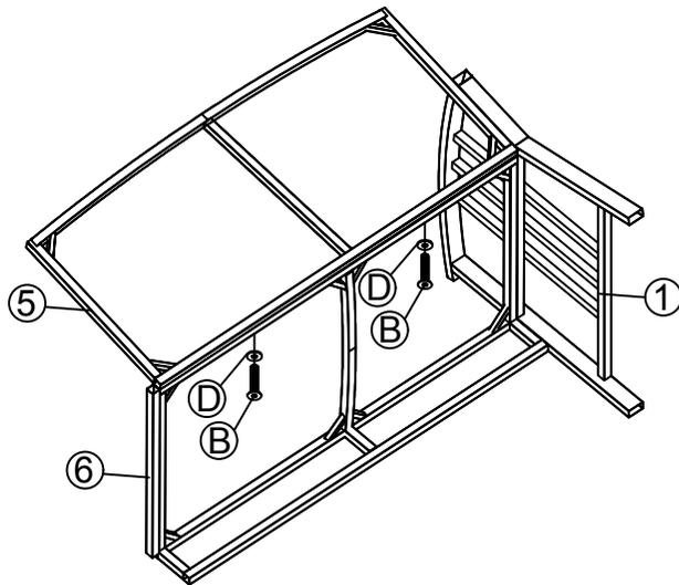
STEP 7: Connect The Part from Step 6 & Back Bench (5), tighten Allen Bolt (A), (B), Flat Washer(D) with Allen Key (E).
