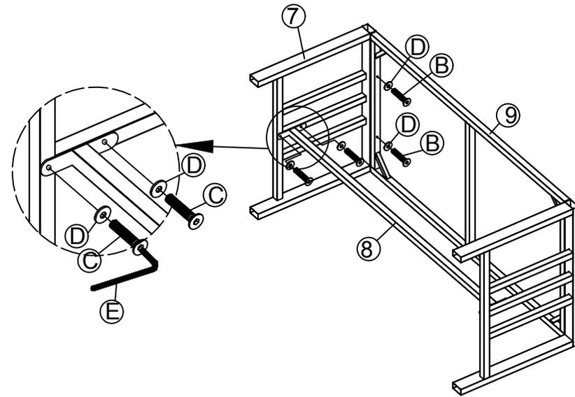
STEP 14: Connect The Part from Step 13 & Leg Table (7), tighten Allen Bolt (B)(C), Flat Washer (D) with Allen Key (E).
