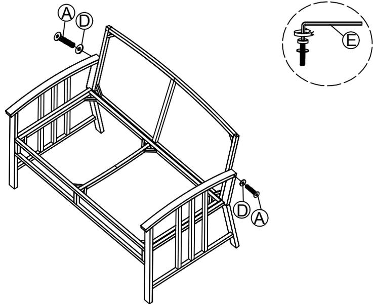
STEP 9: Connect The Part from Step 8 & Left Frame (2), tighten Allen Bolt (A), Flat Washer (D) with Allen Key (E).
