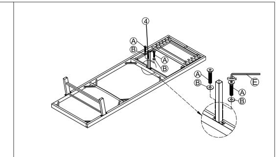
STEP 2: Connect The Part from Step (1) & Middle Leg (4), tighten Allen Bolt (A), Flat Washer (B) with Allen Key (E).
