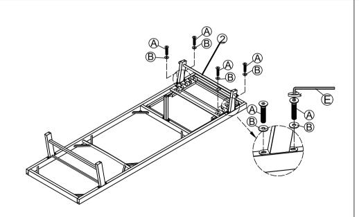
STEP 3: Connect The Part from Step (2) & Front Leg (2), tighten Allen Bolt (A), Flat Washer (B) with Allen Key (E).
