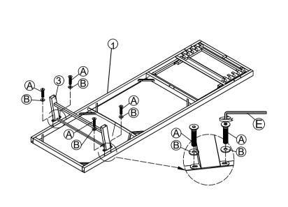
STEP 1: Connect Back Leg (3) & Seat frame (1), tighten Allen Bolt (A), Flat Washer (B) with Allen Key (E).
