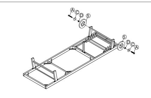
STEP 4: Connect The Part from Step (3) & Wheel (5), tighten Allen Bolt (A), Washer (D), Flat Washer (C) with Allen Key (E).
