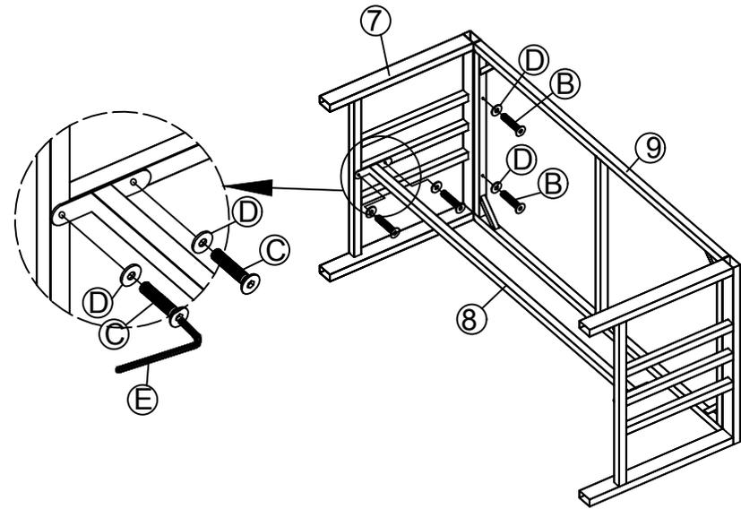
STEP 14: Connect The Part from Step (13) & Leg Table (7), tighten Allen Bolt (B)(C), Flat Washer (D) with Allen Key (E).
