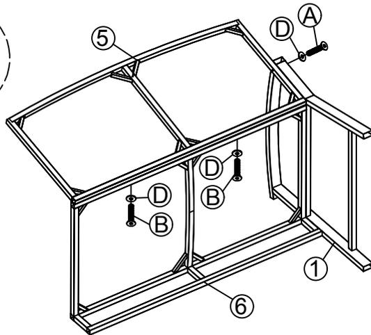
STEP 7: Connect The Part from Step (6) & Back Bench (5), tighten Allen Bolt (A), (B), Flat Washer (D) with Allen Key (E).
