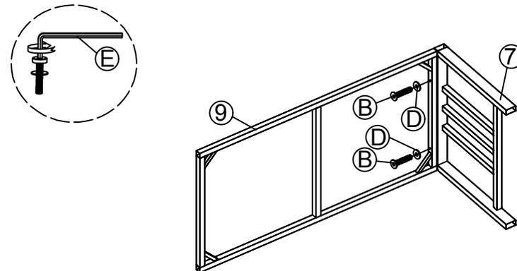
STEP 12: Connect Leg Table (7) & Top Table Frame (9), tighten Allen Bolt (B), Flat Washer (D) with Allen Key (E).
