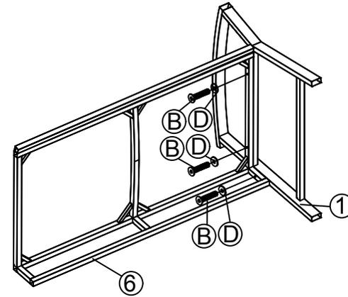
STEP 6: Connect Right Frame (1) & Seat Bench (6), tighten Allen Bolt (B), Flat Washer (D) with Allen Key (E).
