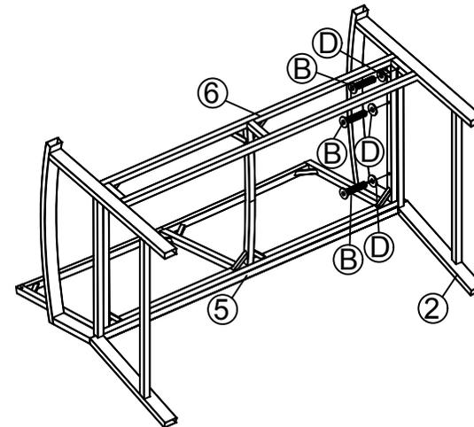
STEP 8: Connect The Part from Step (7) and Left Frame (2), tighten Allen Bolt (B), Flat Washer (D) with Allen Key (E).
