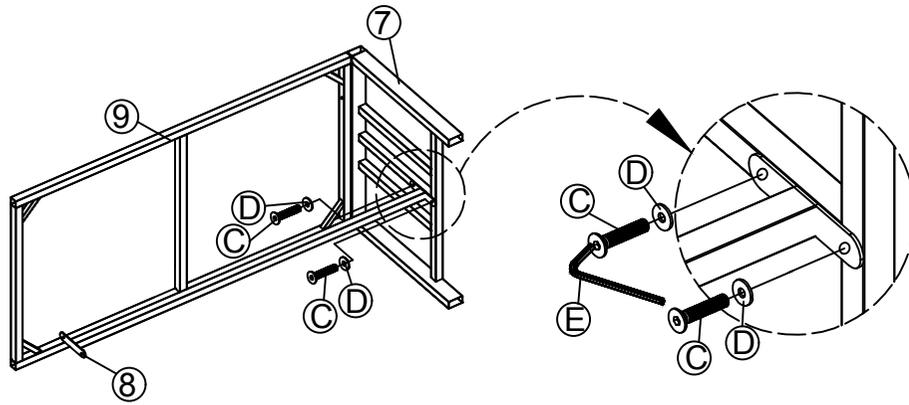
STEP 13: Connect Support Bar (8) & The Part from Step (12), tighten Allen Bolt (C), Flat Washer (D) with Allen Key (E).
