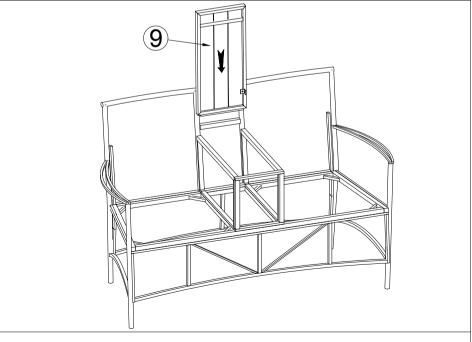
STEP 8: Connect The Part from STEP 7 and Box Top Frame (9).
