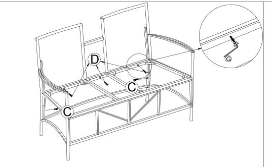
STEP 5: Connect The Part from STEP 4, tighten Bolt (D),(C), Flat Washer (F) with Allen Key (G).
