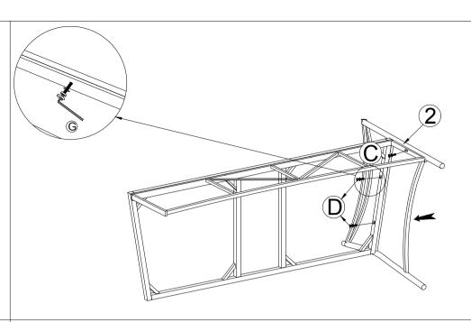
STEP 2: Connect The Part from STEP 1 and Left Frame (2), tighten Bolt (D),(C), Flat Washer (F) with Allen key (G).
