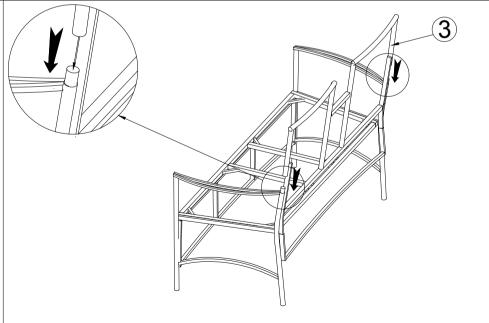
STEP 4: Connect The Part from STEP 3 and Back Frame (3)
