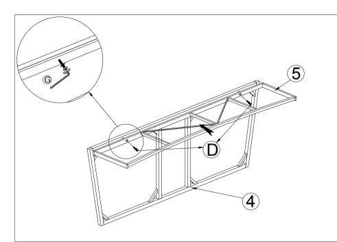
STEP 1: Connect Seat Frame (4) and Front Frame (5), tighten Bolt (D), Flat Washer (F) with Allen Key (G).
