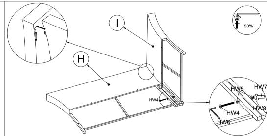
STEP 2: Connect the Part from STEP 1 and Small Back Corner Frame (I), tighten Bolt (HW4), Flat washer (HW5) and Nut (HW8) with Allen Key (HW5) & Key (HW7)
