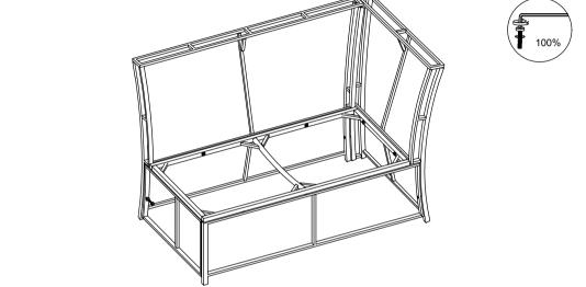
STEP 6: Put the Corner Bench upright and make sure all legs are level, then firmly tighten Bolts with Allen Key (HW6).
