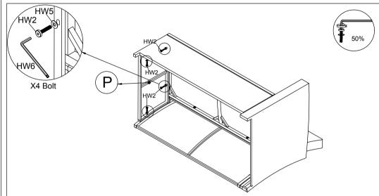
STEP 5: Connect the Part from STEP4 and Right Side Frame (P), tighten Bolt (HW2), Flat Washer (HW5) with Allen Key (HW6)
