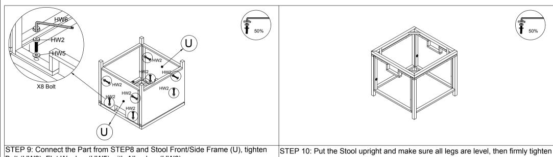
Bolt (HW2), Flat Washer (HW5) with Allen key (HW6).
