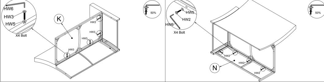
STEP 3: Connect the Part from STEP 2 and Left Seat Frame Frame (K), tighten Bolt (HW3), Flat Washer (HW5) with Allen key (HW6).
