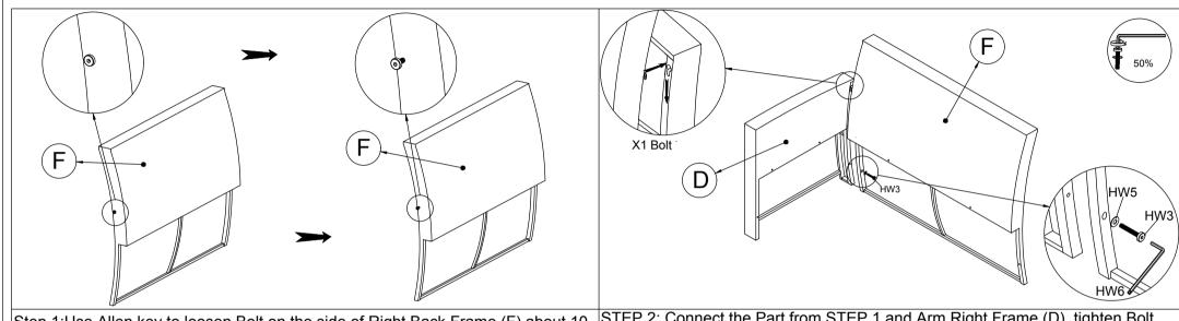
Step 1:Use Allen key to loosen Bolt on the side of Right Back Frame (F) about 10 mm.
