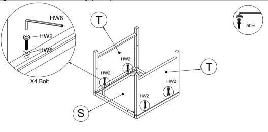
STEP 8: Connect The Stool Seat Frame (S) & Stool Leg Frame (T), tighten Bolt (HW2), Flat Washer (HW5) with Allen Key (HW6).
