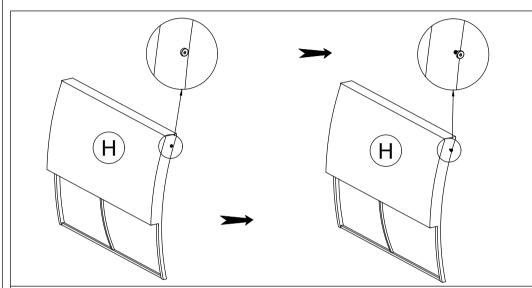
Step 1:Use Allen key to loosen Bolt on the side of Corner Back Frame (H) about 10 mm.
