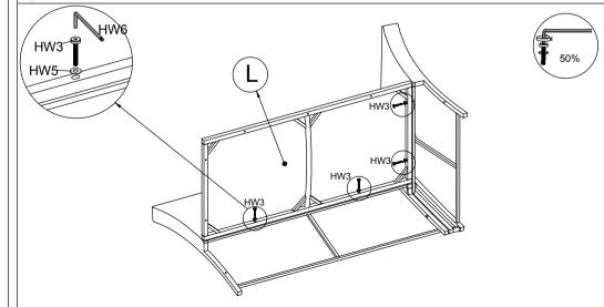
STEP 3: Connect the Part from STEP 2 and Corner Seat Frame (L), tighten Bolt | STEP 4: Connect the Part from STEP 3 and Corner Side Frame (R), tighten Bolt (HW3), Flat Washer (HW5) with Allen key (HW6).
