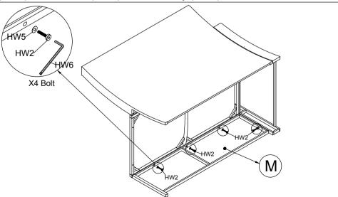
STEP 4: Connect the Part from STEP 3 and Right Front Frame(M), tighten Bolt (HW2), Flat Washer (HW5) with Allen Key (HW6)
