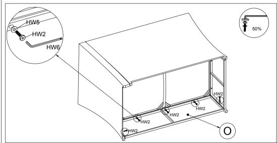
STEP 5: Connect the Part from STEP4 and Corner Front Frame (O), tighten Bolt (HW2), Flat Washer (HW5) with Allen key (HW6)
