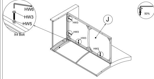
STEP 3: Connect the Part from STEP 2 and Right Seat Frame Frame (J), tighten Bolt (HW3), Flat washer (HW5) with Allen key (HW6).
