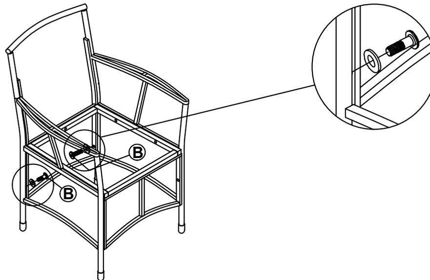
**STEP 5** : Connect the Part from STEP4 and Bolt (C) with Allen key (E).
