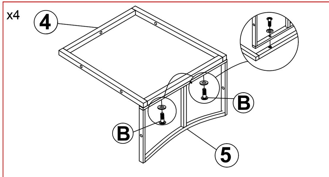
**STEP 1 :** Connect Chair Seat (4) and Chair Front Panel (5), tighten Bolt (B), Flat washer (D) with Allen key (E).
