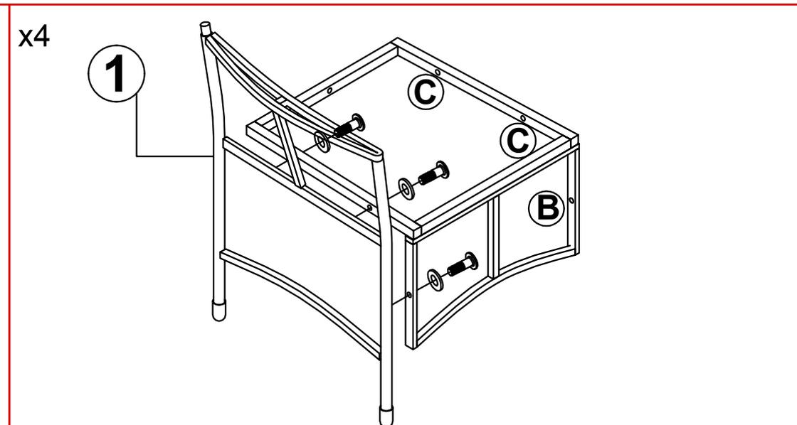
**STEP 1 :** Connect Chair Seat (4) and Chair Front Panel (5), tighten Bolt (B), Flat washer (D) with Allen key (E).
