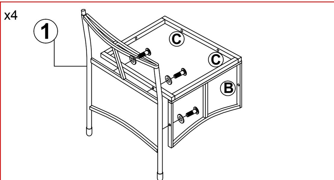
**STEP 2 :** Connect the Part from STEP 1 (4) and Right Frame (1), tighten Bolt (B),(C), Flat washer (D) with Allen Key (E).
