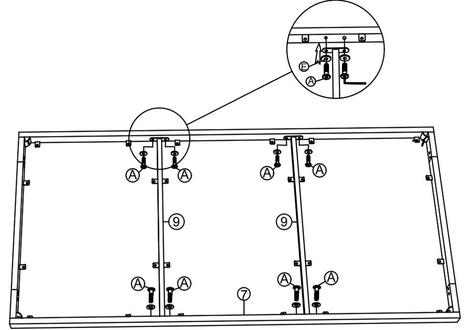
STEP 2 : Connect The Part From STEP 1 and Middle Table Top (9) ,tighten Bolt (A), Flat washer (D) with Allen key (E).
