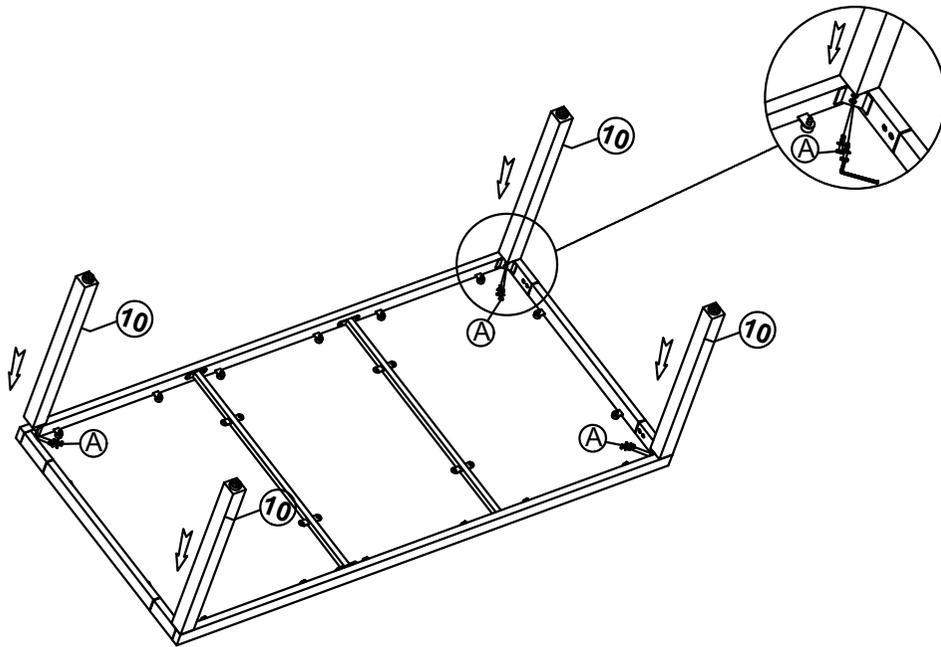
STEP 3 : Connect The Part from STEP 2 and Table Leg (10), tighten Bolt (A), Flat Washer (D) with Allen key (E).
