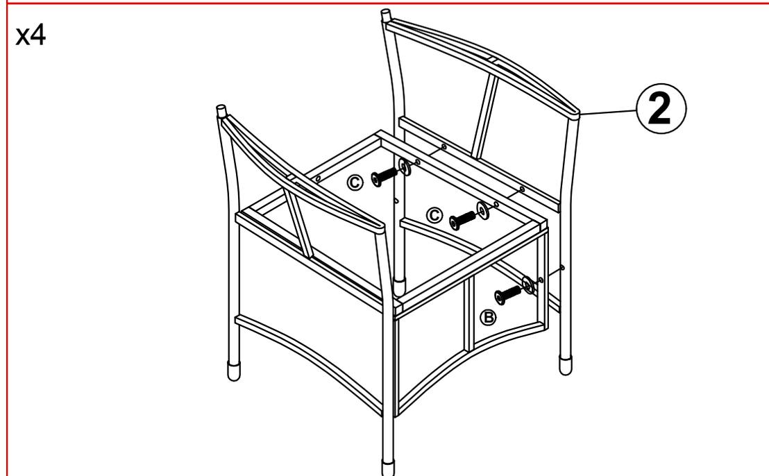
**STEP 3 :** Connect the Part from STEP 1 (4) and Left Frame (2) tighten Bolt (B), (C), Flat washer (D) With Allen key (E).
