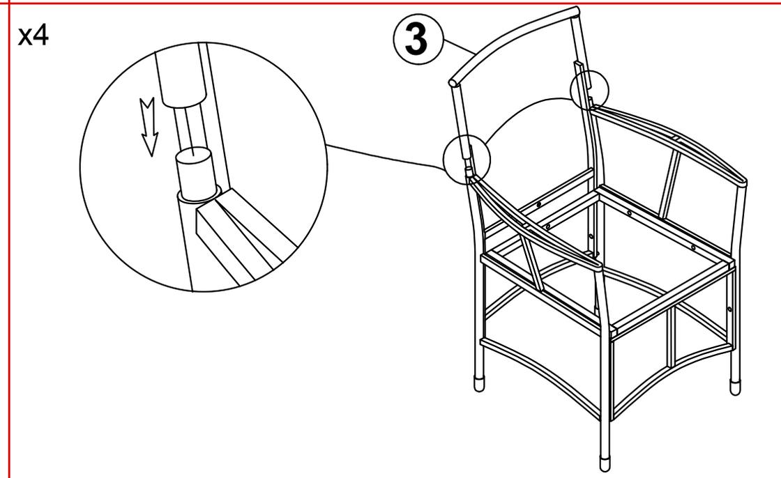
**STEP 3 :** Connect the Part from STEP 1 (4) and Left Frame (2) tighten Bolt (B), (C) Flat washer (E) With Allen key (F).
