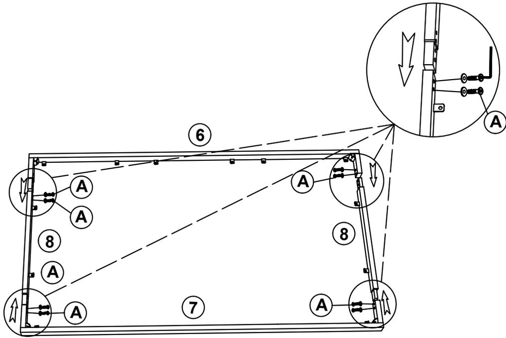
STEP 1 : Connect Long Table Top Frame 1 (6) with Short Table Top Frame (8), Long Table Top Frame 2 (7) with Short Table Top Frame (8), tighten Bolt (A), Flat washer (D) with Allen key (E).
