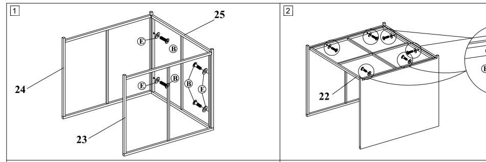
Step 1 Connect Corner Right Frame (25) & Corner Front Frame (23), Corner Back Frame (24) & tighten Bolt (B) with Allen key (F)
