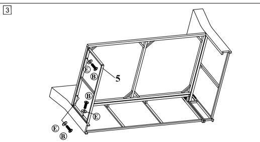
Step 3 Connect part from Step 2 & Bench Side Frame (5) tighten Bolt (B) with Allen key (F)
