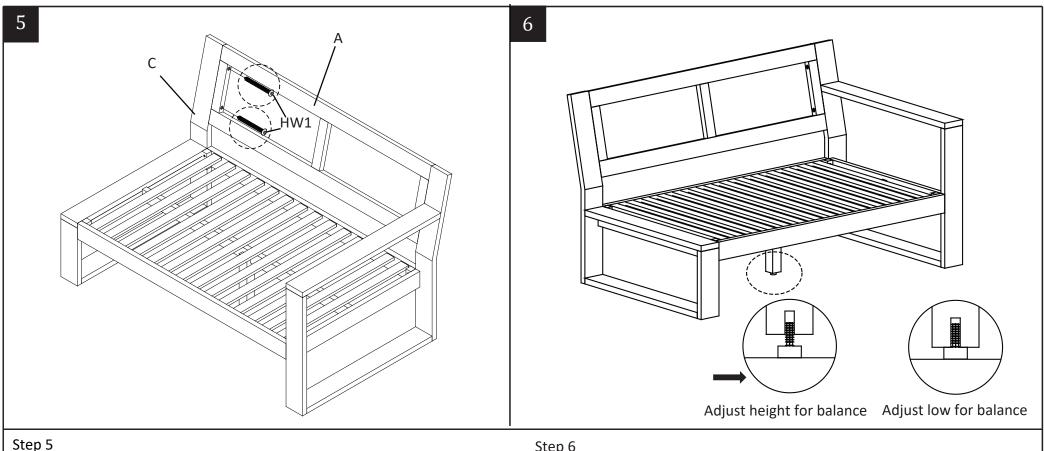
Tighten Screws (HW1) with allen key (HW4) to attach Back Frame (A) and leg frame -1 (C)
