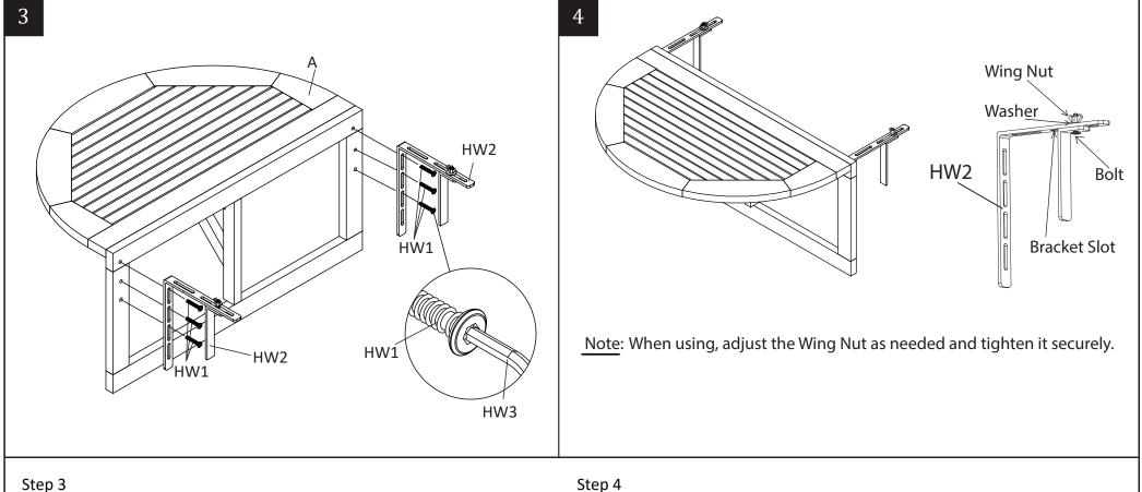
Attach Pass hang the balcony table (HW2) to leg frame Balcony table (A). Use Bolts (HW1) ,tighten with allen key (HW3).
