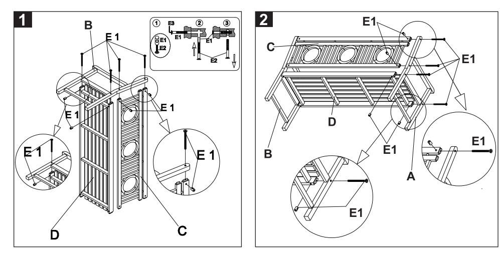
Step1: attach the left side (B) to the back (C) and the seat (D) as shown on the picture by using the Allen bolt (E1). Tighten all with the Allen key (E3).
