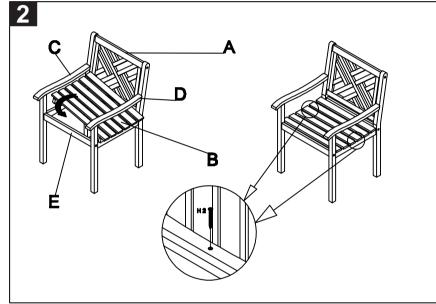
Step 1: attach left side (D) to the back (A). Then attach the supports (E) as shown on the picture by using the Allen Bolt (H1) and tighten it with the Allen Key (H4). Continue with the right side (C) in the same way. Make sure to tighten all bolts (H1) before You continue with step 2.
