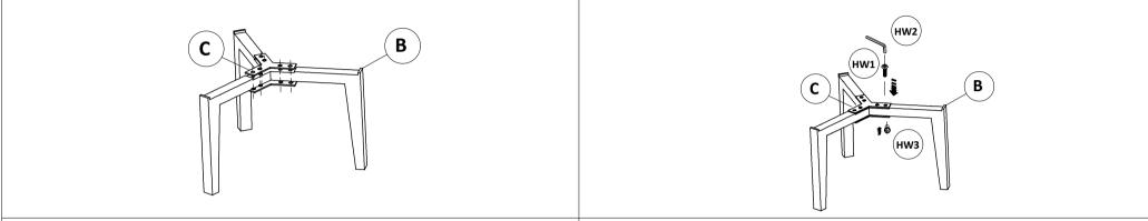
**STEP 1:** Use bracket (C) to fix the wooden legs: one bar above and one bar below so that 6 holes of the bracket (C) are concentric with the 6 holes available on the wooden legs.
