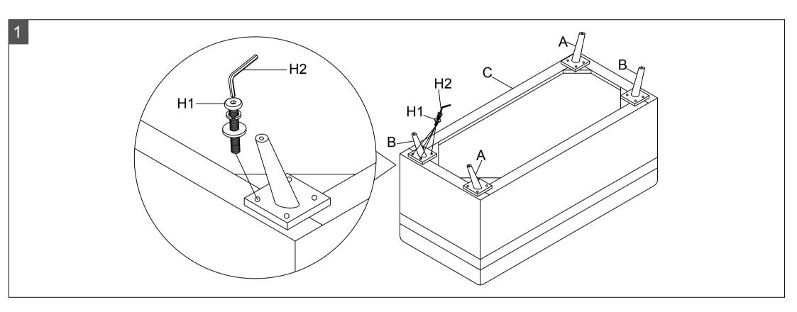
Step 1: Attach 4\*legs (A&B) to the corresponding position on the underneath of cabinet by using Allen key (H2) to lock with 16\*Allen bolts (H1), as picture.
