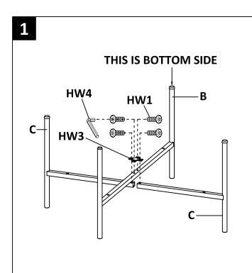
\*Do not fully tighten the bolts until the product is assembled.
