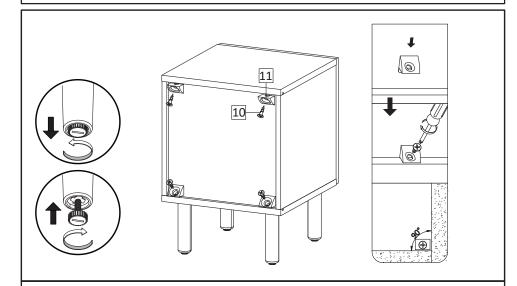
**STEP8**: Use Wedge (HW11), Screw M 3.5 x15.5 (HW10) to tighten the back of night stand by using screwdriver. Please align the top board and bottom board in  $90^{\circ}$  position againt the side board, before securing the wedges (HW11).
