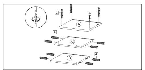
**STEP1**: Insert Cambolt (HW1)into Top Board (A). Insert Dowel (HW4) into Side Board Left (C) and Side Board Right (D).
