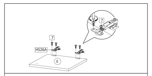
**STEP6**: Insert Hinge (HW HS26A) into pre-hole in Wooden Door (E). Secure with Screw M4.5 x12.5 mm (HW7).
