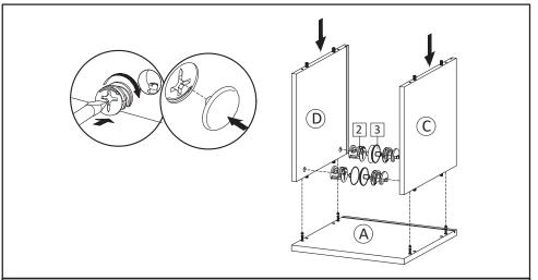
**STEP2**: Attach Side Board Left (C) and Side Board Right (D), into Top Board (A). Insert Camlock (HW2) then tighten using screwdriver.
