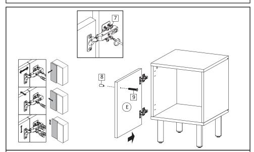
STEP7: Install Wooden Door (E), into Side Board Left. Secure with Screw M4.5 x 12.5 mm(HW7). Please refer to the last page for more guide on how to adjust hinges.
