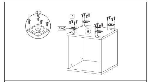
**STEP4**: Install Mounting Plate (PM2) and secure with screw M4.5x12.5mm (HW7) on Bottom Board.
