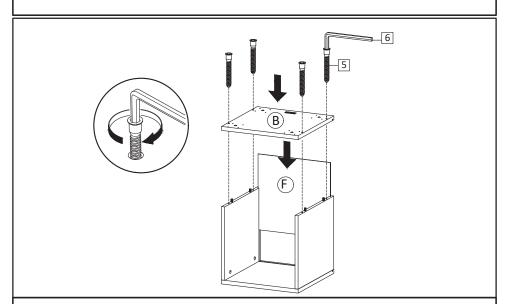
**Step3**: Insert Back Board (F) as figure. Put Bottom Board (B) and secure with Screw M7x50 (HW5), tighten screws using Allen Key (HW6).
