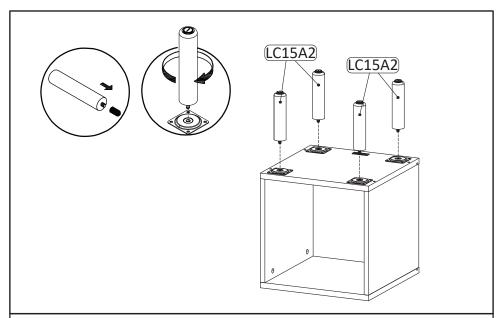
**STEP5**: Insert Leg (LC15A2) into Mounting Plate, tighten by rotating . the leg clockwise.
