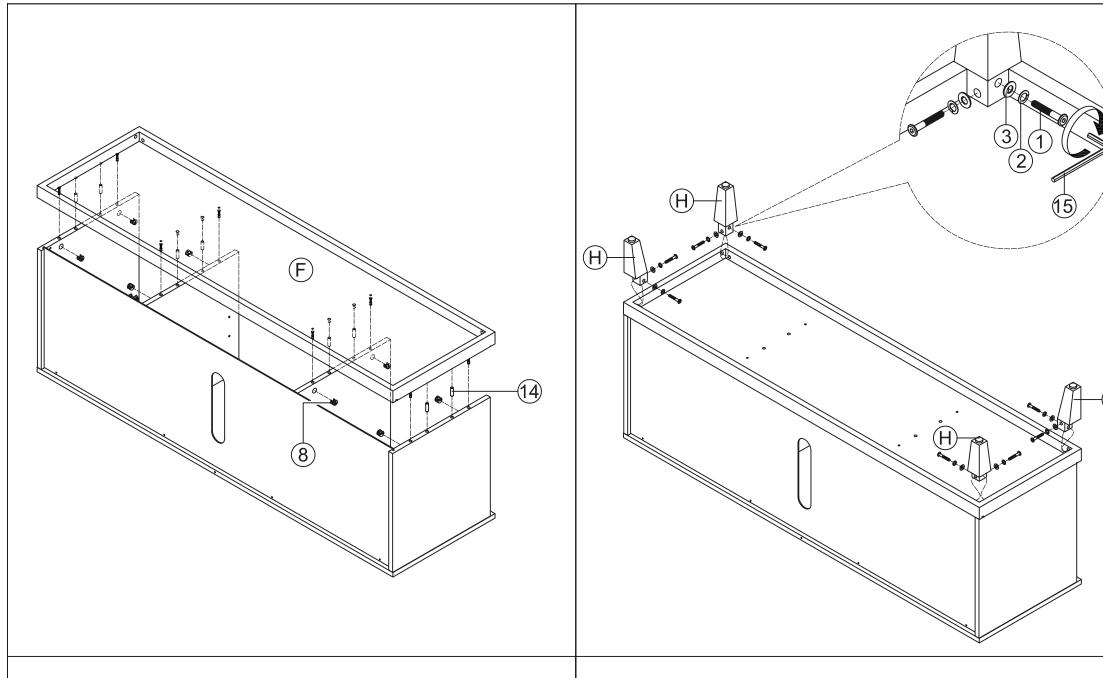
STEP 7 ATTACH BOTTOM PANEL TO UNIT USING CAM LOCKS AND DOWELS.
