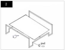
Sten 2 Put the marble top (B) on the base(C) carefully, tighten the screws (C)
