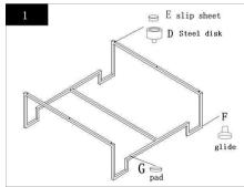
Step 1 Put 4 glides (F) under the legs of the base(C) Put 6 slip sheet  $\,(E)\,$  on the top of steel disk  $\,(D)\,$  ,then Put the steel sheet  $\ (D)$  on the top of the base  $\ (C)$
