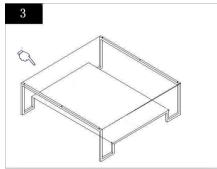
Sten 3 Put the glass top (A) on the base(C) carefully, Check if the top (A) (B) match the base (c) perfectly. The assembly is finished
