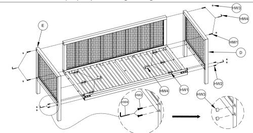
STEP 3: Attach the armrest-1 and the armrest-2 as illustrated in picture. Make sure to apply all the bolts into the holes properly before tightening.
