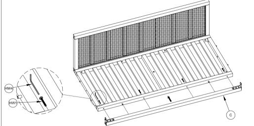
STEP 2:Attach the horizontal brace to the seat frame. Make sure to apply all the bolts into the holes properly before tightening.
