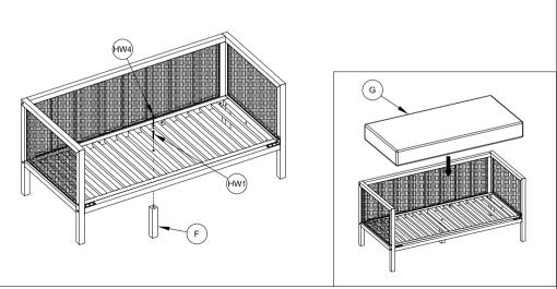
STEP 4: Attach the center leg as illustrated in picture. Make sure to apply the bolts into the holes properly before tightening.
