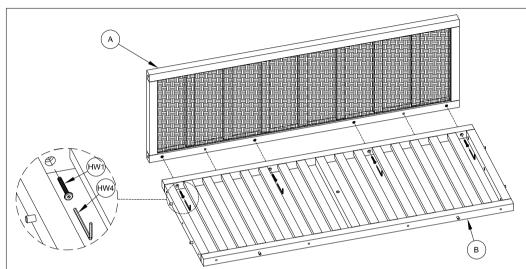
STEP 1: Attach the seat frame to the back frame. Make sure to apply all the bolts into the holes properly before tightening.
