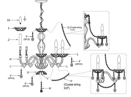
**Step 6:** Place socket cover(J), glass bowl(I) and bulb(H) to the lampholder.
