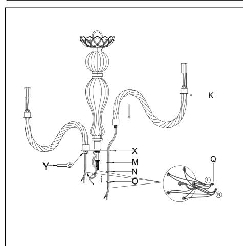
**Step 1:** Place the glass arm(K) to the metal round plate(X) and tighten with washer(M), spring washer(N) and thick hex screw(O), secure the thick hex screw (O) balance the 5 arms evenly with spanner (Y).
