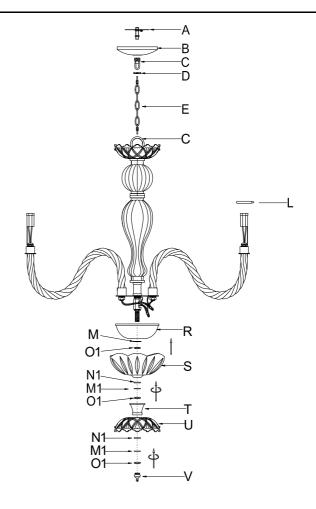
Step 2: Place the support wire cap(R), internal teeth washer(M), thin hex screw(O1), glass bowl(S), plastic washer(N1), flat washer(M1), thin hex screw(O1) and trumpet cap(T), glass bowl(U) to the nipple of the metal round plate(X) then tighten with plastic washer(N1), flat washer(M1), thick hex screw(O1) and metal finial(V). Place acrylic ring(L) to the glass arm(K) by cross the lampholder. Screw the chain(E) to the lock(C) of the lampbody
