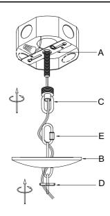
**Step 5:** Place Lock(C) to mounting bracket and then secure chain(E) to Lock(C). Attach the Canopy(B) to the junction box and fix it by turning the Canopy Nut(D) clockwise.
