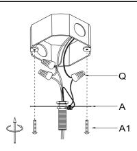
**Step 4:** Install the Mounting Plate(A) to the junction box with Mounting Screw (A1).
