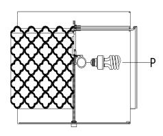
PLEASUE USE ON/OFF TYPE"B" BULB MAX 60-WATT OR CFL BULB MAX 13-WATT THERE ARE 3PCS CFL 13 -MATT BULB IN THE BOX
