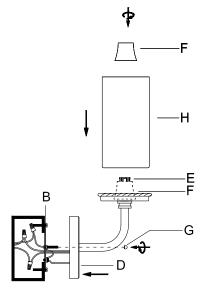
Insert the bulb (I) into the Socket(E). Be sure to use the bulb with wattage not exceed than specified on the fixture.
