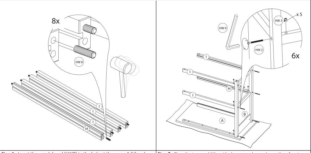
**Step 1:** Insert the wood dowel (HW8) to the hole at the apron 1 (H) and apron 2 (I).
