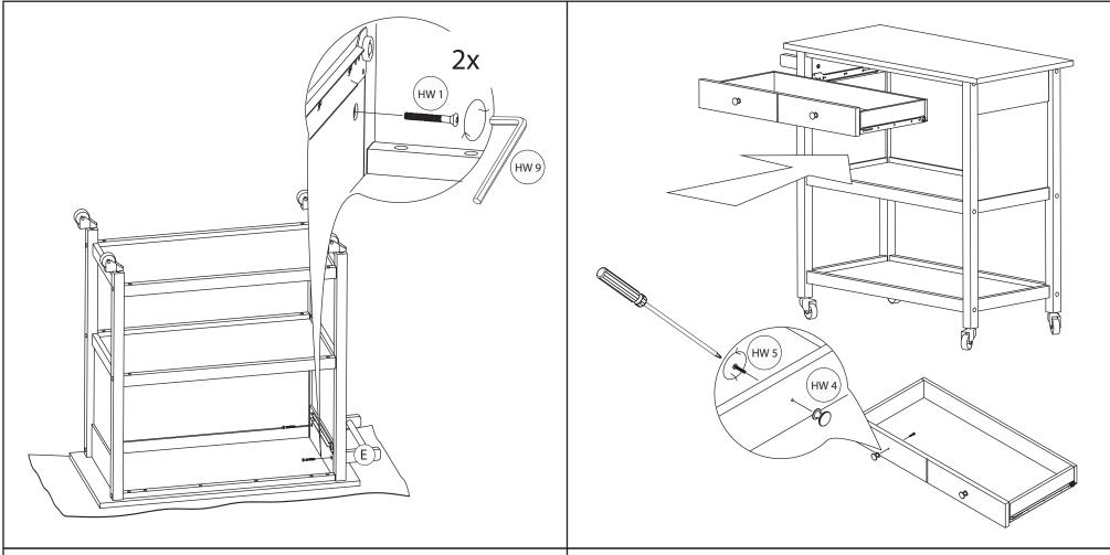
**Step 5**: Assemble the handle bar (E) to the leg frame L (B). Tighten the handle bar (E) using the screw (HW1).
