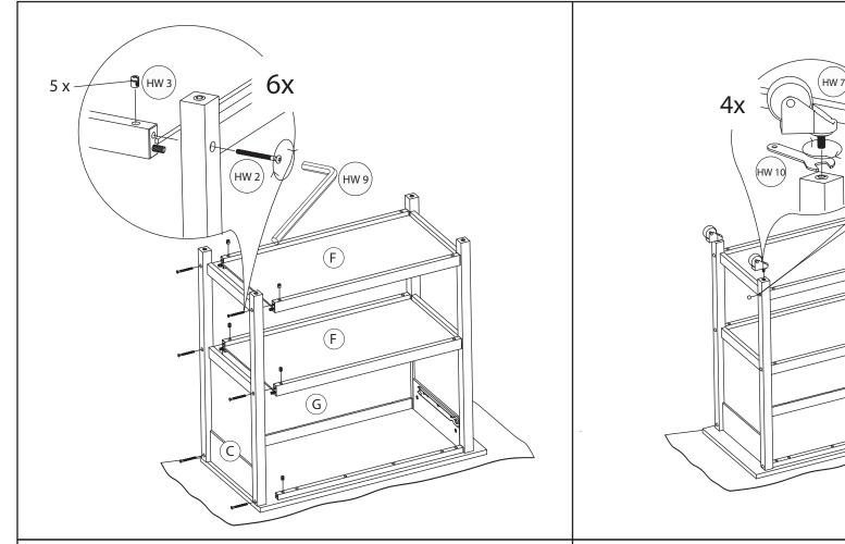
**Step 3 :** Insert shelf (F) into the groove of apron (H) and apron (I). Attach leg frame R to all of the aprons. Insert nut (HW3) at the first hole of the apron and tighten it with screws (HW2).
