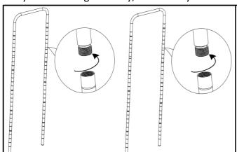
STEP 1: SCREW BOTH HANDLES(C) INTO THE POLES(B) BY SCREW CONNECTORS ASSEMBLED ON HANDLES.
