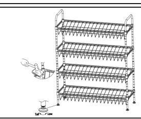
STEP 6: PUSHING FIRMLY DOWN ON EACH SHELF AT ITS CORNER OVER PLASTIC CLIPS AND SCREW LEVELING FEET TO ATTAIN PROPER LEVELING.
