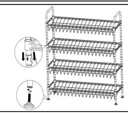
ISTEP 4: SET THE RACK UPRIGHT. PRESS THE SHOE ISTEP 5: REFER TO STEP 3&4 TO ASSEMBLE THE FIRSTLY. THEN SCREW LEVELING FEET(E) INTO BOTTOM OF POLES.
