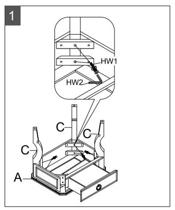
Step 1: Attach 3 legs (C) first, screw with cabinet (A) by using Allen key (HW2) to lock with 6\*bolts (HW1)
