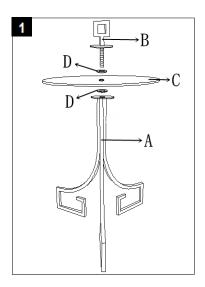
Step 1: Assemble the Leg (A) Clear washer(D) Top glass(C) Finial(B) together as shown in the picture .
