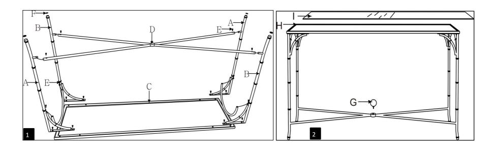
Upside down the top frame on ground, attach legs and shelf together Use allen key to tighten all bolts
