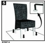
Leveling FRONT legs until the chair become standing stable and then fasten all screws tightly FULL with Allen key (E4).
