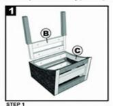
Align front leg (B) onto the bottom of seat base (C)
