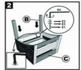
STEP 2 with seat base (C). Attach front leg (B) using Allen bolt (E1), Spring washer (E2) and Flat washer (E3). Fasten HALF TIGHT with Allen key (E4) onto 4 hol
