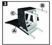
STEP 3 bled front leg (B) and seat base (C) onto the backrest (A). Adjust the position to fit perfectly.
