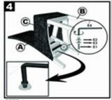
STEP 4 Attach assembled front leg (B) and seat base (C) onto Backrest (A) using Allen bolt (E1), Spring washer (E2) and Flat washer (E3). Fasten HALF TIGHT with Allen key (E4) onto 4 holes for
