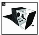
STEP 6 Put bottom cover by pressing the edges of fabric to volcro fixed. Stand up the chair upright. Assembly is
