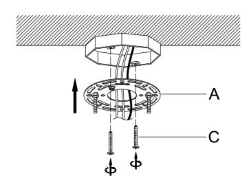
**Step 4:** Fix the Mounting Plate(A) to the junction box with Mounting Screw (C).
