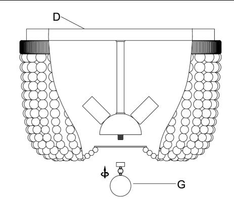
**Step 2**: insert the hole in the iron plate below the lamp body (D) into the threaded part of the junction box. The figure shows the iron plate at the bottom of the lamp body. Turn Finial (G) clockwise until tightened.
