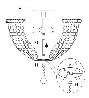
**Step 2**: Fix one end of Tube(G) to the Lamp Body(D) in a clockwise direction, Place the iron frame below the Lamp Body (D) on the threaded part of the Tube (G). The iron frame at the bottom of the lamp body is shown in the figure. Turn the Finial (H) clockwise until tight.
