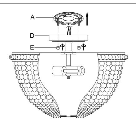
**Step 1**: Unpack all parts from cartons carefully. Turn the Canopy Nut (E) counterclockwise to separate the Mounting Plate (A) and Lamp Body (D).
