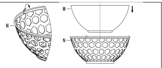
**Step 2:** Place the glass (M) in the hollow lamp shade(N), and fix the glass inside with clip to make it firm according to the drawing
