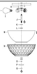
**Step 6:** Twist the nipple (J) on the suction canopy (G) On the nut below, cover the glass (M) and hollow-out lamp shade(N) on the nipple (J) according to the drawing, and then use the nex nut (O) to cover the steel ring (K) glass and washer (L) is locked on the nipple (J). Then cover the central pipe and lock the finial (Q) as shown in the picture
