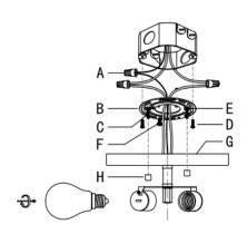
**Step 5:** Attach the Canopy (G) through Mounting Screw (C), secure Canopy (G) with Finial (H) to Mounting Screw (C). Lock the bulb (I) into the socket
