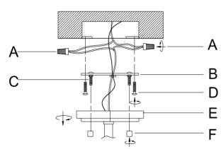
**Step 3:** Using the Wire Nut (A) connected the positive electrode and the negative pole of the fixture body carefully into the positive electrode and the negative pole in junction box.
