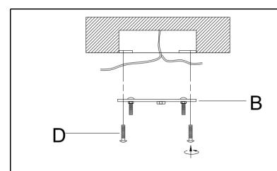
**Step 1:** Attach the Mounting Plate (B) to the junction box using the Outlet Box Screw (D) on the ceiling wall.
