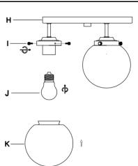
**Step 4:** Install the bulb (J) onto the lamp body (H), and tighten the glass cover (K) onto the lamp body (H) with the decorative nut (I).
