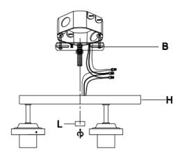
Step 3: Fix the lamp body (H) to the mounting bracket (B) with the decorative nut (L).
