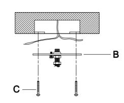
**Step 1:**Attach the Mounting Plate (B) to the junction box using the Outlet Box Screw (C) on the ceiling wall.
