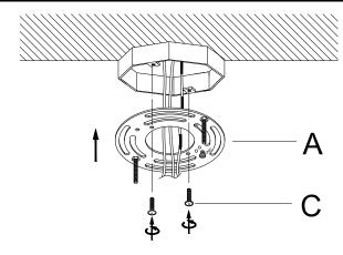
**Step 3:** Insert the J-box wires through the center opening of Mounting Plate (A). Attach the Mounting Plate (A) onto the J-box and secure it by turning the 2 Mounting Screws (C) clockwise until tight.
