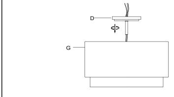
**Step 2**:Insert the fixture wires through the Canopy (D). Rotate the Canopy (D) clockwise till tight.
