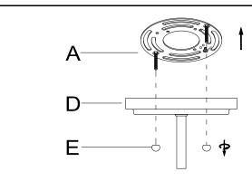
**Step 1:** Unpack all parts from cartons carefully. Separate the Mounting Plate(A) from the Canopy(D) by removing the Canopy Nut(E) anti-clockwise.
