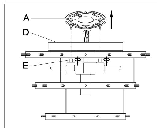
**Step 1**: Unpack all parts from cartons carefully. Turn the Canopy Nut (E) counterclockwise to separate the Mounting Plate (A) and Lamp Body (D).
