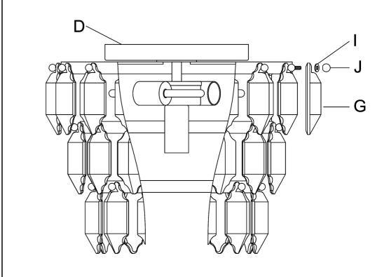
**Step 2**:Place the hole of the Crystal (G) on the exposed thread of the Lamp Body (D) .Then put on the Rubber Pad(I). rotate the Ball Nut (J) clockwise to hold it in place. Repeat this action. Load from the bottom to the top until all the crystals are covered.
