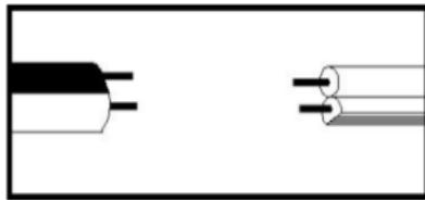
\*Note: When parallel wire(SPTI&SPTII)is used. The neutral wire is square shaped and ridged and the hot wire will be round in shape and smooth.(See illustration on left)
