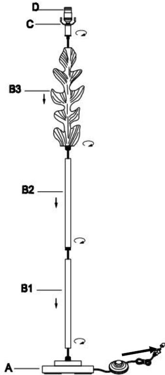
**Step1:** Screw the Saddle(C) and socket (D) onto the Lamp body(B3). Screw the Lamp body (B3) onto the Lamp body(B2). Screw the Lamp body (B2) onto the Lamp body(B1). Screw the Lamp body (B1) onto the Lamp base(A). Be careful not to twist the power cord and tighten securely.
