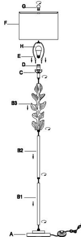
**Step2:** Insert the Harp (E) into the Saddle (C). Put the shade (F) on the Harp (E), then tighten the Finial (G) into the Harp (E). Insert the bulb (H) into the socket (D).
