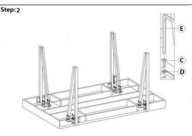
Please keep all screws loose and tighten TOGETHER after assembling.
